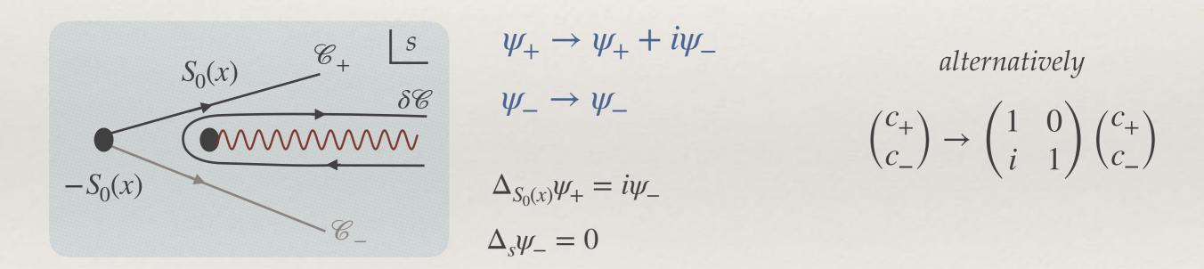
Strategy: 1) Analyze the Stokes phenomena around each turning point to construct locally2) Patch the local solutions to construct the global wave-function.
